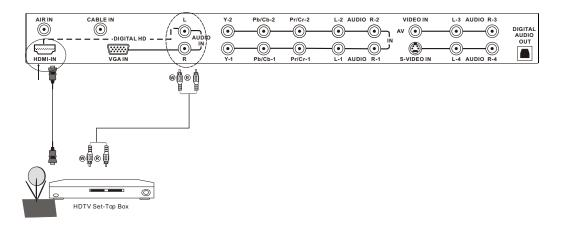
1. Turn off the power to the LCD TV and HDTV Set -Top Box.
